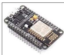
Figure 4-4: NodeMcu development board
