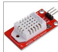
Figure 4-5: DHT22 Temperature and humidity sensor
